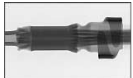
Microfocus X-ray image of a crimp about 2 millimeter in diameter. Counting the strands helps to understand the limitations of a conventional X-ray inspection. Photo: phoenix|X-ray Systems + Services Inc.
